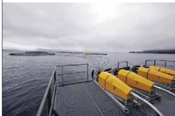
PLATE 113 Feed delivery pipes connecting the centralized feed system with the cages
