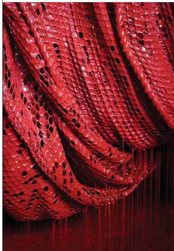
PLATE 78 Net dipping in an antifoulant tank
