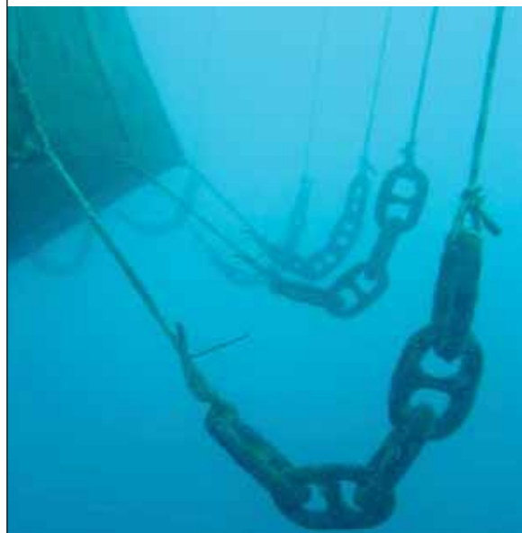
PLATE 34 Stud link chains used as sinkers. Chains are preferable for use as net tensioning ballasts because of the greater weight in water of steel, compared with concrete, stones or other materials
