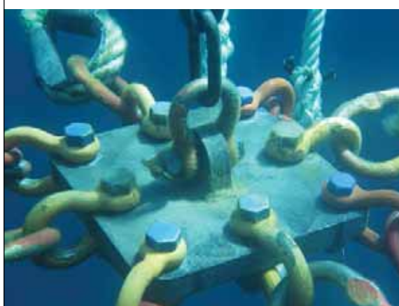
PLATE 14 Corner plate, eight holes. Four are used to connect the main mooring lines; four are used to connect paired mooring bridles for the cages
