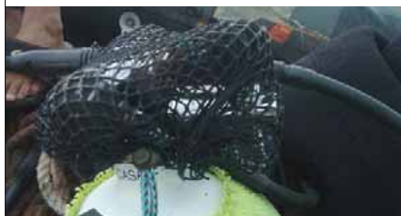
PLATE 124 Protective cover made of knotless netting is wrapped around the first stage of a scuba diving regulator to reduce the risk of it becoming entangled in the seine net
